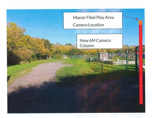
The proposal for mounting the CCTV surveillance camera within the Manor Fields Play Area would be to install a new 6m column and associated power. Note there is currently a disconnected mains feeder pillar located adjacent to the allotments which could provide the main power to the new column.
