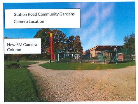
The proposal for mounting the CCTV surveillance camera within the Station Road Community Gardens area would be to install a new 5m column and associated power. Note there is currently a mains feeder located within the adjacent council-owned Men's-Shed building. (approx. 5m soft dig)
